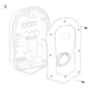
Remove all 8 screws from the enclosure and carefully lift away.
