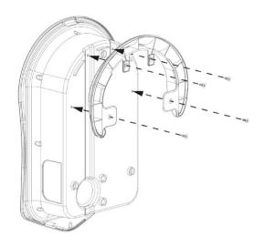
If installing a tethered zappi, you must ensure the cable wall guard is fixed to the unit using the 4 screws supplied.
