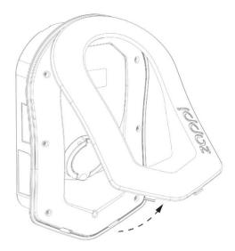
Carefully remove fascia from the **zappi** by pressing the 2 clips located at the bottom of unit inwards whilst pulling the fascia towards you.
