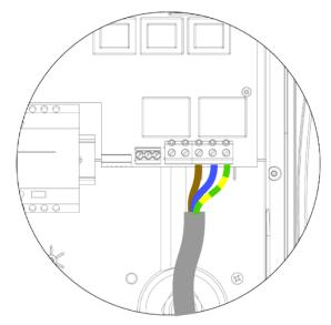
For single-phase installations, without the need for hardwiring an external CT, please follow the above diagram
