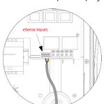
Connect the eSense cables using the diagram
