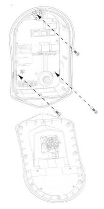
Secure the unit to the wall using the fixing kit provided. Ensure the grommets are used to maintain its IP integrity.
