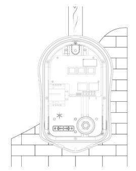
Using **zappi** template mark mounting holes. For fixing to brick, use the top and 2 bottom holes (left/right). Use the 2 vertical holes as well as the top hole if mounting to a stud wall or joist.
